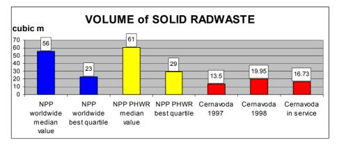
FIG. 4. Solid Radwaste Generation
